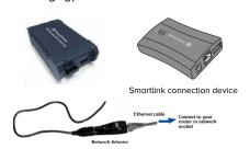
Reconnect at home by plugging your network cable with adapter into one of the yellow LAN connectors at the back of your broadband router (not the red WAN connection).
